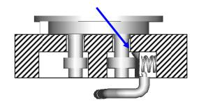
No axial moving parts are required to generate the required pull force onto the lamp. This simplifies the design and increases the reliability.
