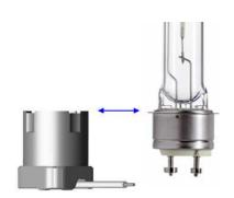
The lamp can be inserted into the lampholder without any force until the flange of the lamp cap touches the upper rim of the barrel of the holder. After the lamp cap is sitting on the lampholder barrel, the lamp can be twisted clockwise until a mechanical stop. A snap-insensation confirms proper insertion of the lamp.
