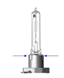
The patented contacts of the lampholder contain slopes on the top edges. During the rotation of the lamp the slopes create an axial force onto the boss of the lamp pins. This force pulls the lamp securely down into the lampholder. The spring loaded contact is designed to compensate the tolerances of the ceramic housing of the lampholder and the pins of the lamp.
